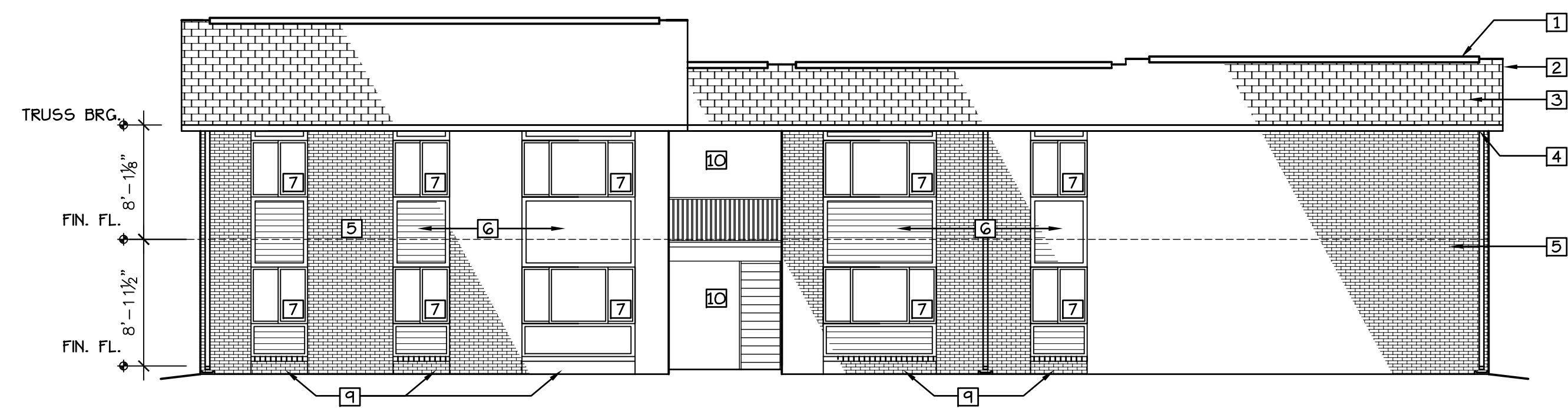
BLDG'S '1','4','6','7' REAR ELEVATION SCALE: 1/8"=1'-0"
