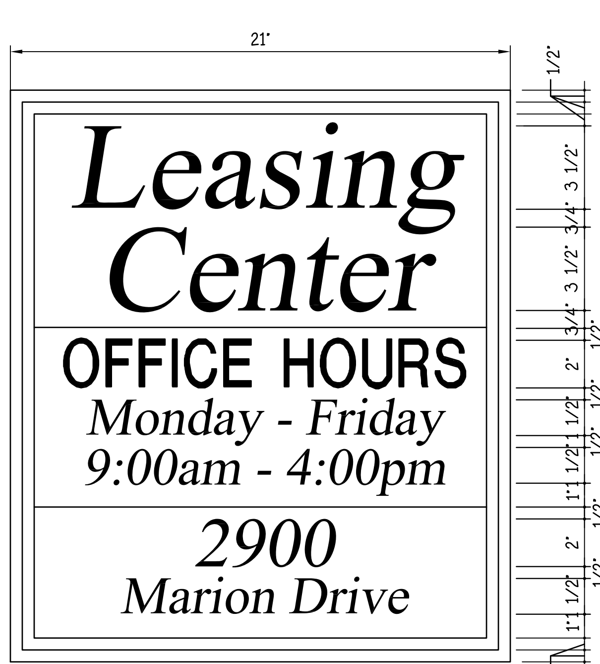
(C1) - 21x24. SINGLE-SIDED SIGNFOAM. HDU SANDBLASTED WOOD GRAIN BACKGROUND.
