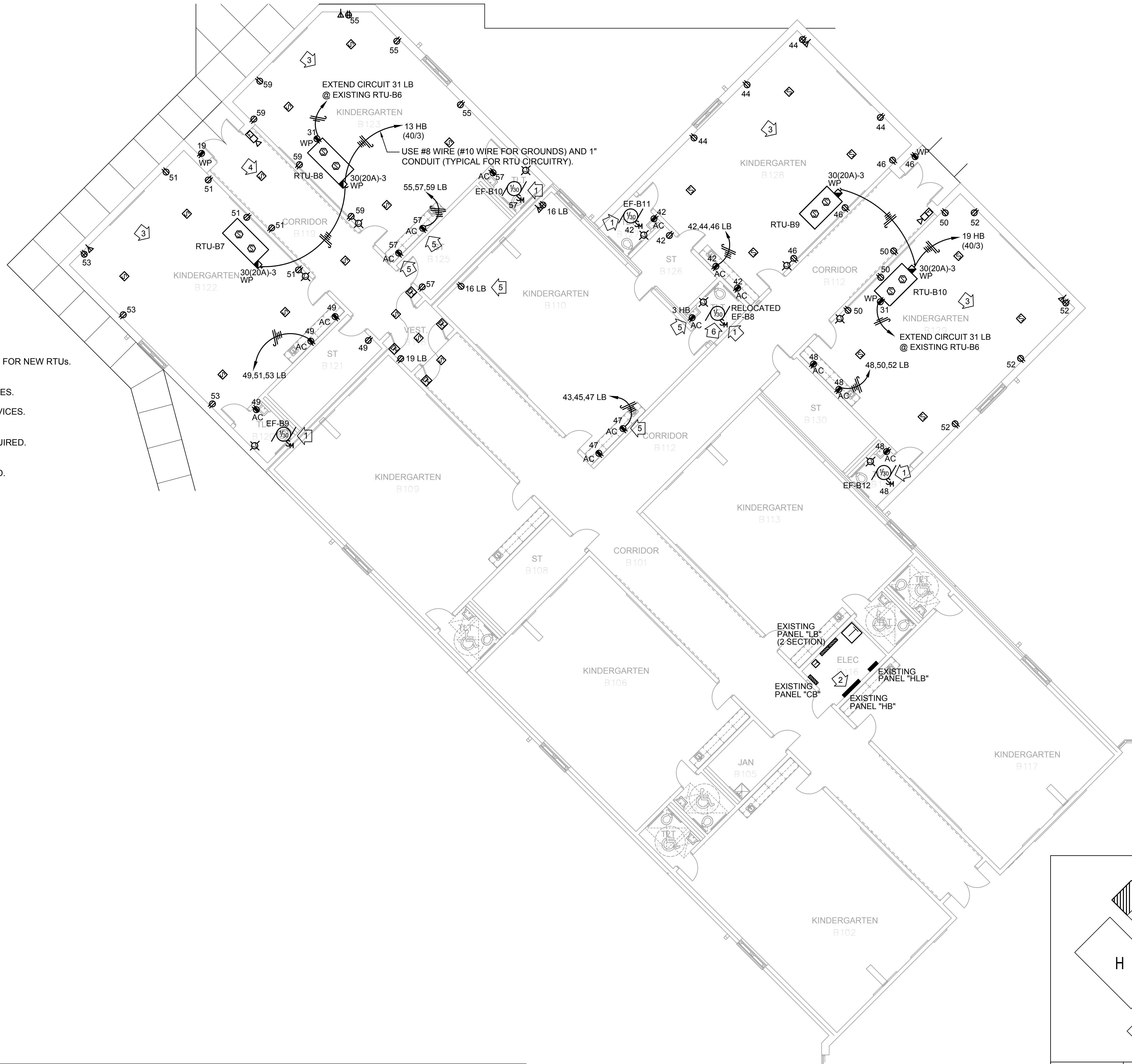
A1 PARTIAL FLOOR PLAN - AREA B POWER & FIRE ALARM - ELECTRICAL 1/8"=1'-0"
