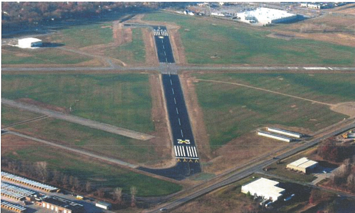
Figure 2-1 Markings for a Temporarily Closed Runway
