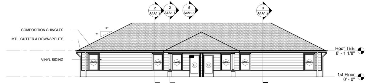
**8 WEST ELEVATION - BUILDING 2B2A**
