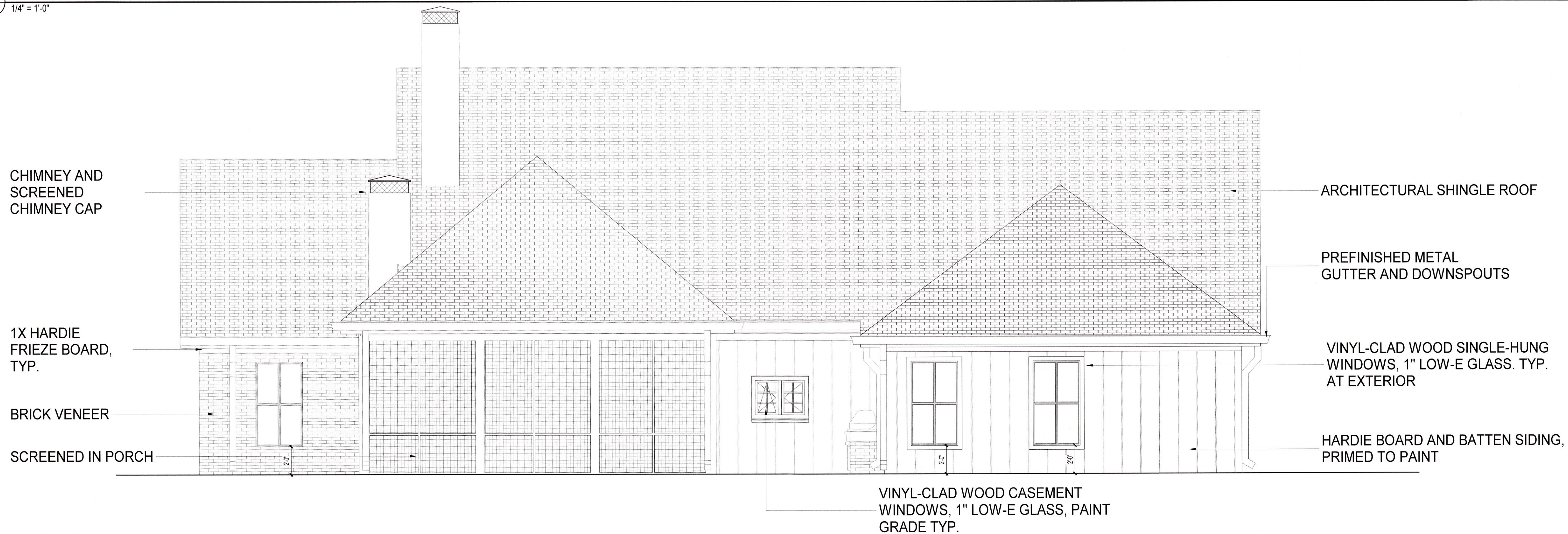
1 NORTH ELEVATION A3.1 1/4" = 1'-0"
