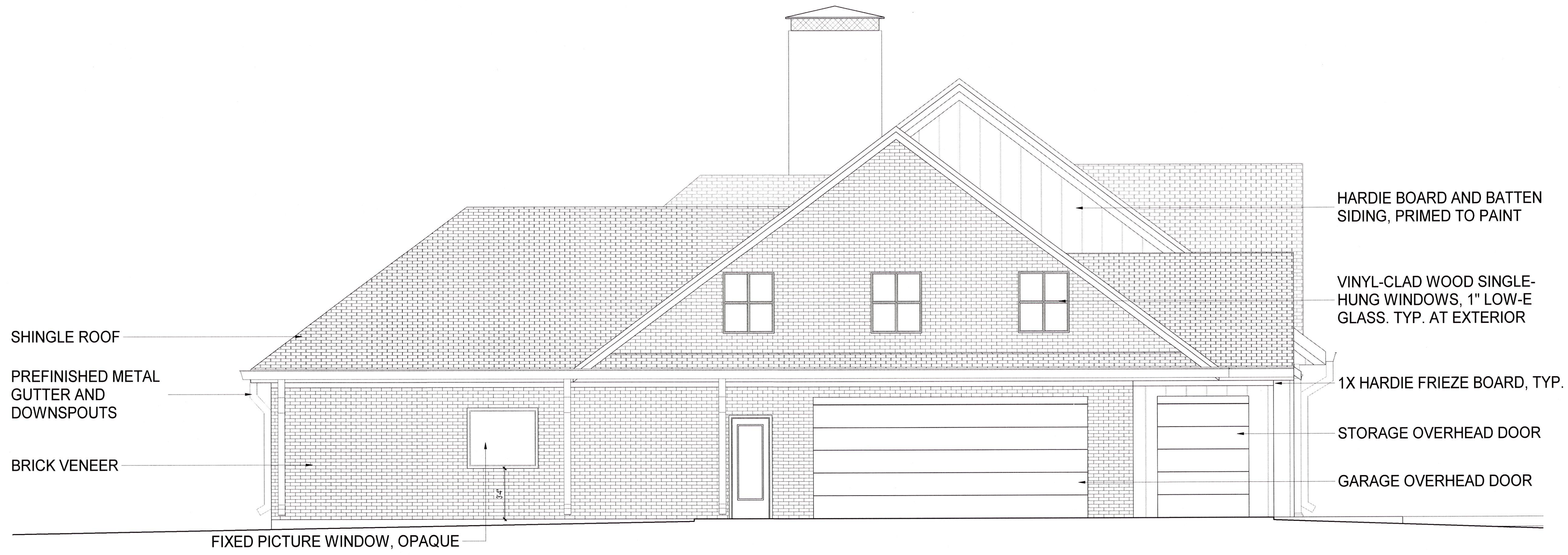
1 WEST ELEVATION A3.2 1/4" = 1'-0"
