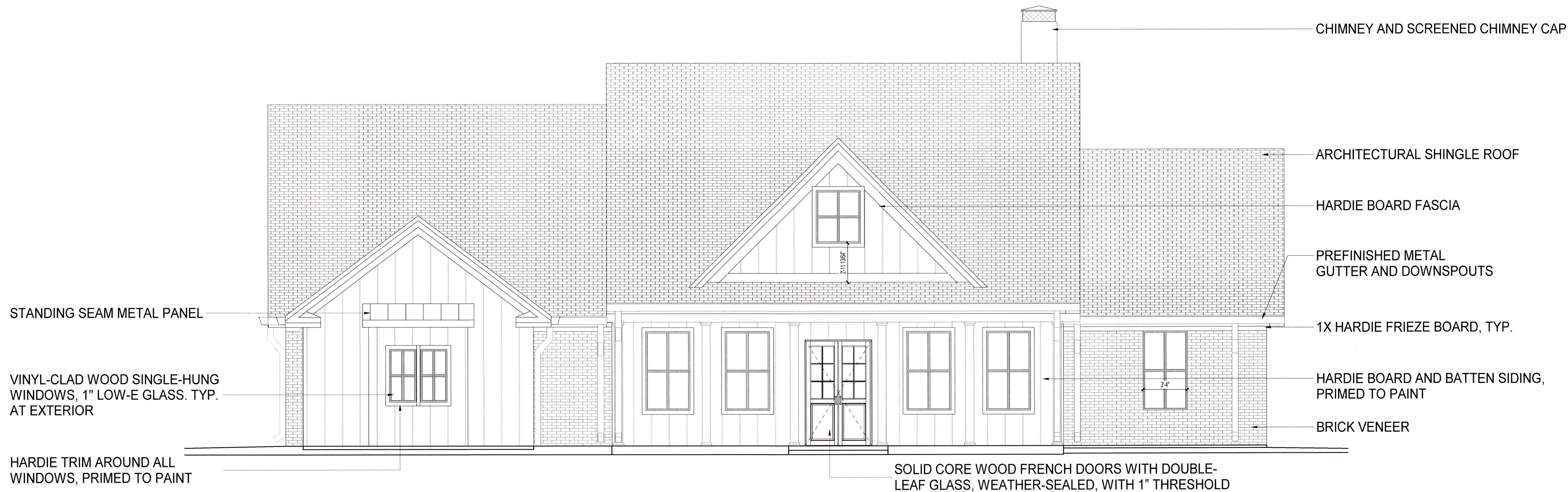
2 SOUTH ELEVATION A3.1 1/4" = 1'-0"
