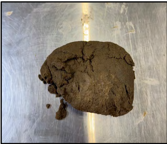
Figure 5: Stratum III SM material from B-02 encountered at approximately 13.5 feet below the existing surface elevation.
