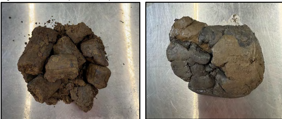
Figure 3: Stratum II CL material from B-02 encountered at approximately two (2) feet below the existing surface elevation.
