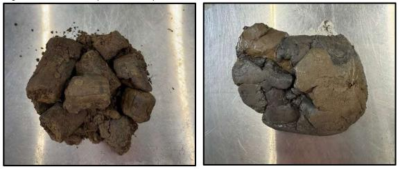
**Figure 3:** Stratum II CL material from B-02 encountered at approximately two (2) feet below the existing surface elevation. **Figure 4:** Stratum II ML material from B-01 encountered at approximately 18.5 feet below the existing surface elevation.
